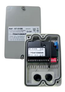
**HF receiver** with built-in antenna and two relays (07-0106).
